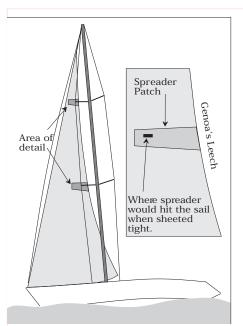
All Mylar-based genoas either come with spreader patches in place or with spreader patch material to be applied. The patches are sticky-back Dacron material that protect the sail from wear as the sail scrapes across the ends of the spreaders during a tack. <u>Never use a genoa without the patches in place.</u>
